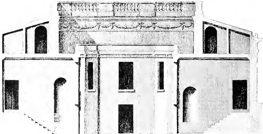
Section of the Hot Bath at BATH, the Design of John Wood, Architect.
